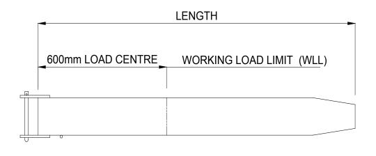
Bremco's Forklift Extension Slippers allow you to temporarily lengthen the tynes of your forklift for load stability and are ideal for large crates or machinery items.
